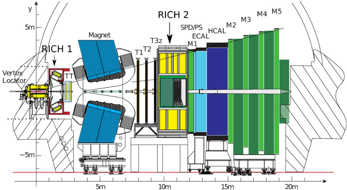
Figure 1. The LHCb Detector, highlighting the two RICH detectors (Fig. 1 from [5]).
