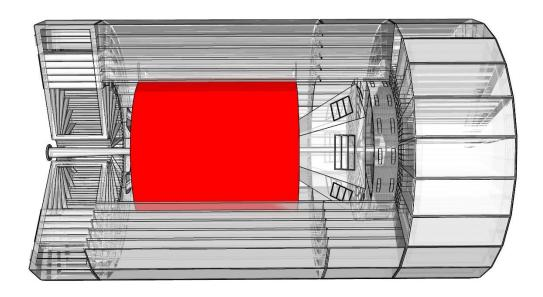
Figure 5: Solenoid Cryostat
