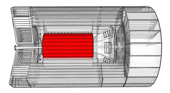
Figure 7: Barrel Electromagnetic Calorimeter
