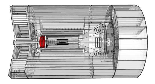
Figure 9: Lepton Direction Electromagnetic Calorimeter
