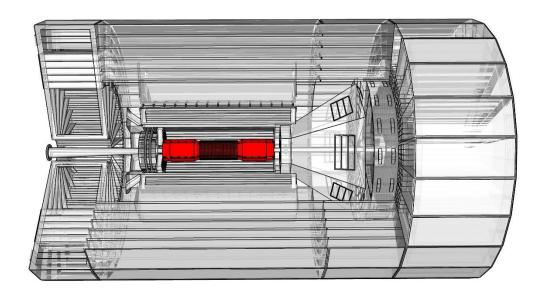
Figure 14: Silicon Vertex Detector
