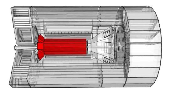
Figure 8: DIRC Detector
