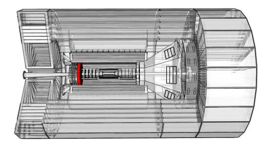
Figure 10: Lepton Direction Time of Flight Detector
