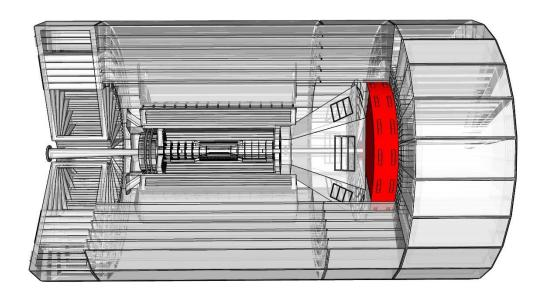
Figure 13: Hadron Direction Electromagnetic Calorimeter
