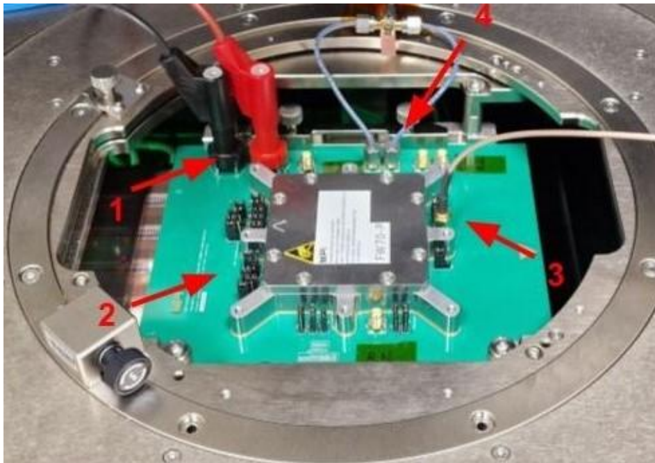
Figure 3. Serializer (NKF7) vertical probe card, where 1 - power connectors, 2 - configuration jumpers, 3 - Clock, 4 - differential output
