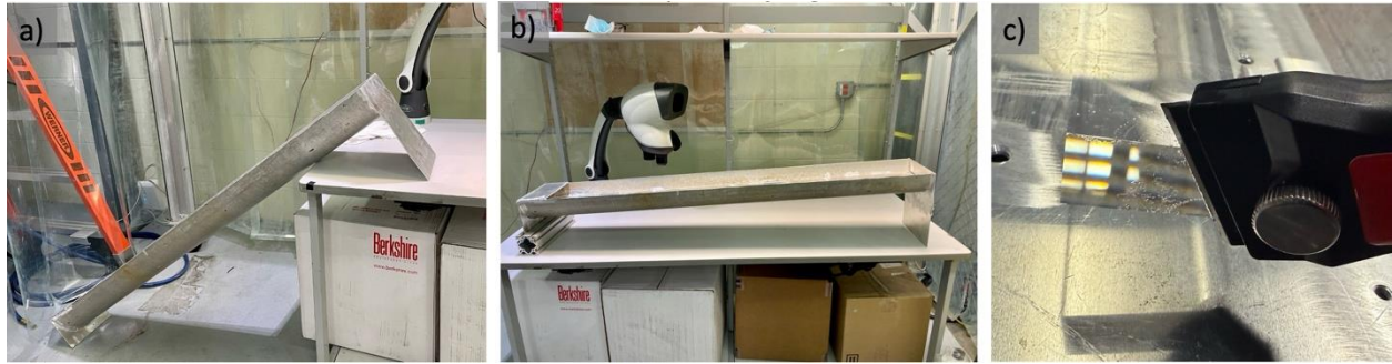
Figure 2. Photos of the setup used to remove residue glue from separated DIRC bars.
