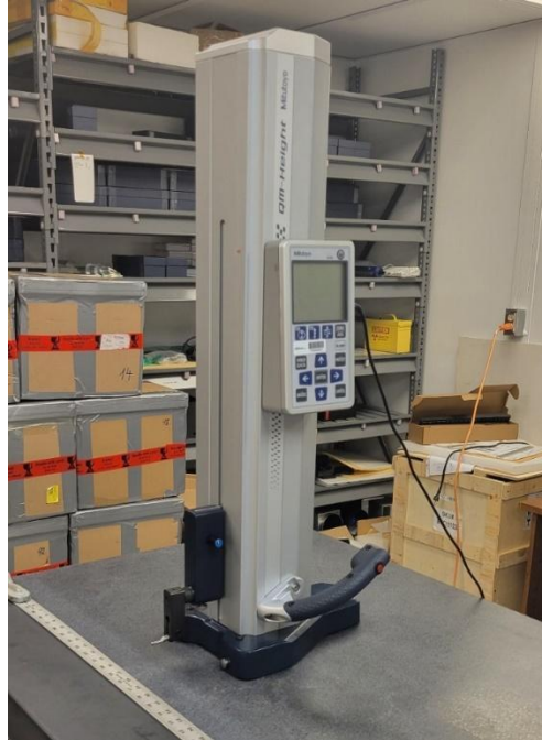
Figure 3. The Mitutoyo QMH-14" B digital height gauge in the NPS Clean Room on the granite slab table.
