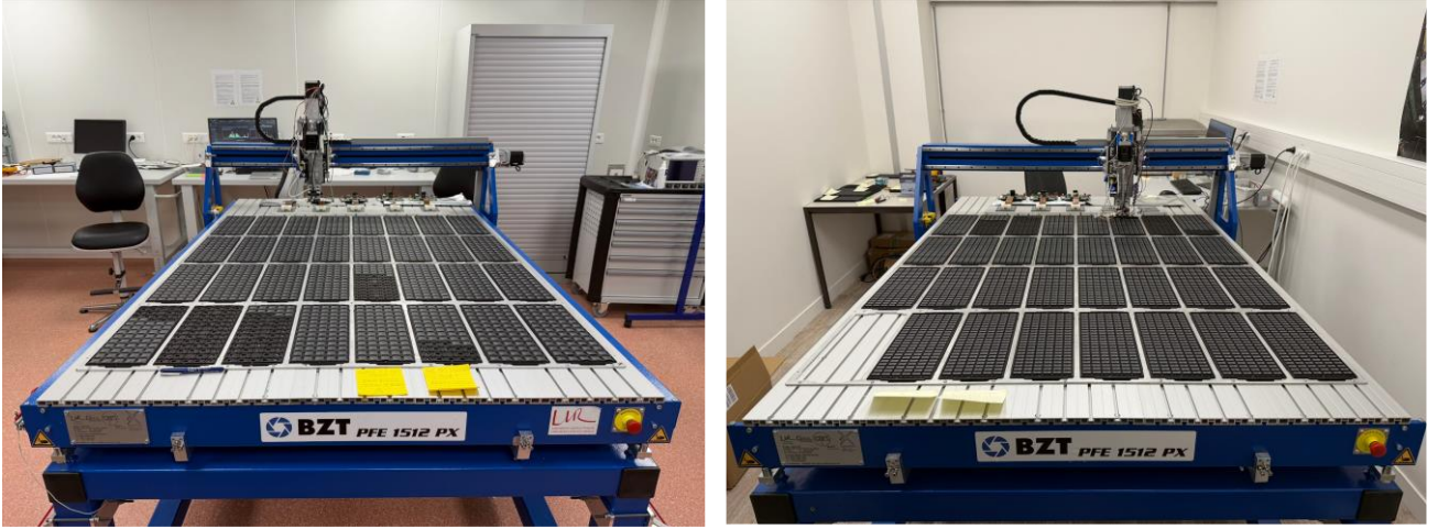
Figure 1. Robots used for qualifying HGCROC HD packages (left) and LD packages (right).
