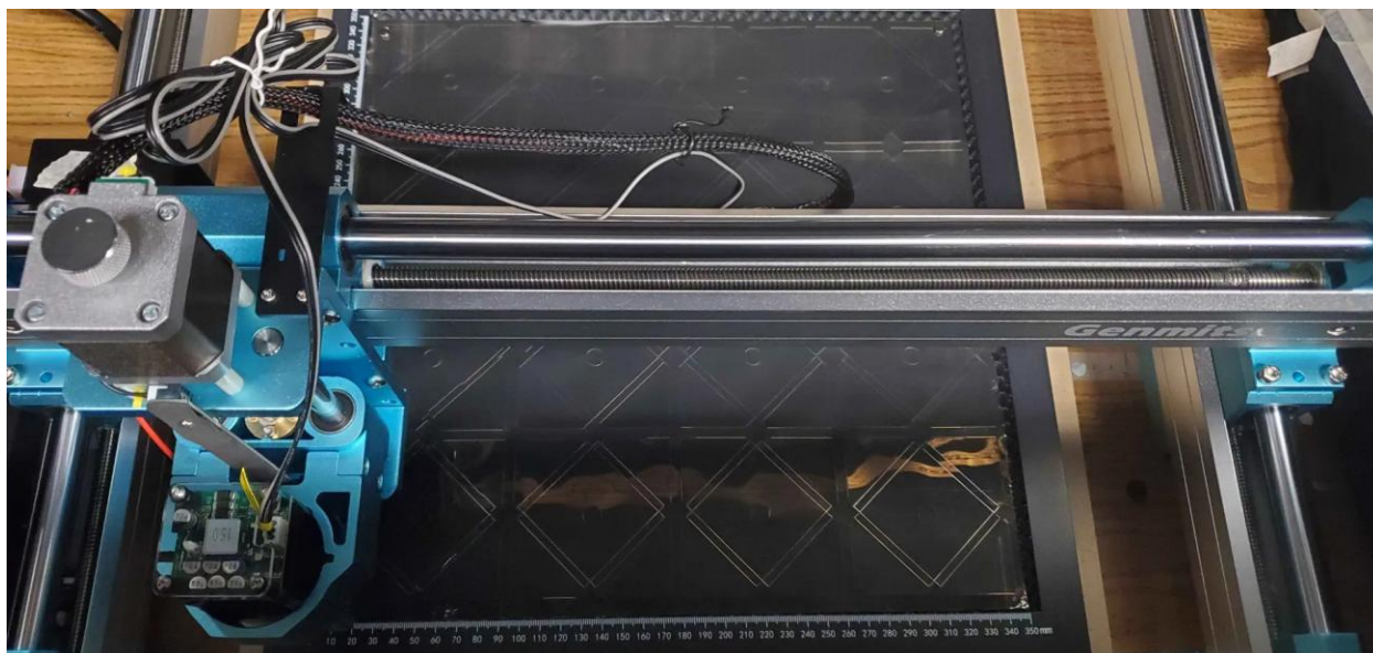
Figure 2. CNC 500 mW Laser Cutter, cutting a 400 cm x 400cm sheet of ESR Foil
