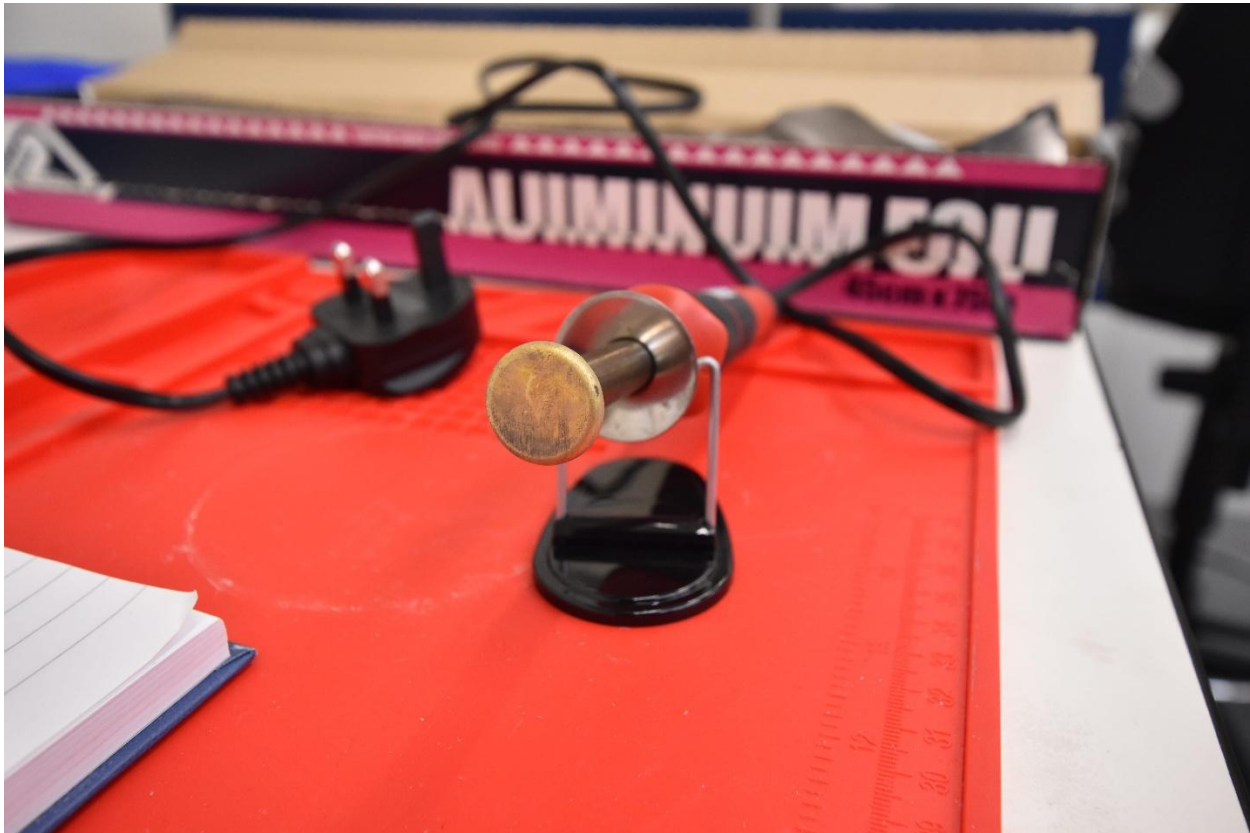
Figure 3. An example heat source used to melt fiber ends.
