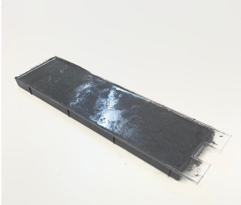
Figure 16. Top view of a finished module after removal from the mold.
