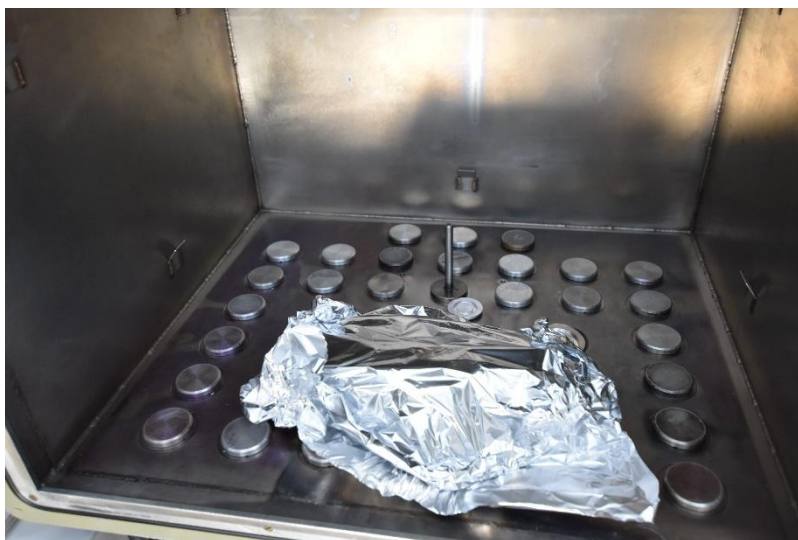
Figure 13. Mold loosely wrapped in foil placed in a vacuum chamber.
