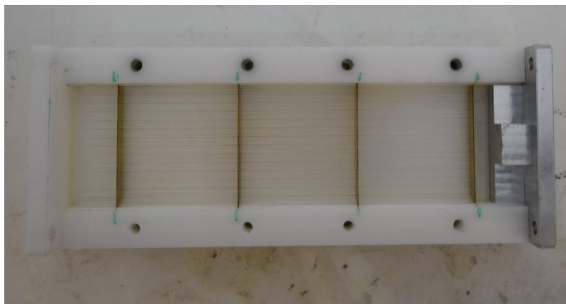
Figure 8. A fiber matrix successfully inserted into the mold. Note the green markings showing clearly the location of the mesh slots as mentioned in step b).
