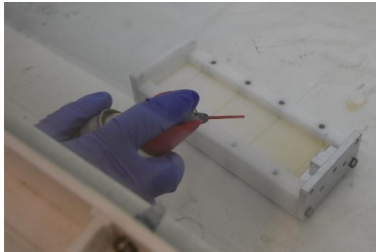
Figure 6. PTFE spray being applied to the inside surfaces of the mold.
