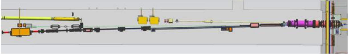
Figure 20. Preliminary CAD rendering of the Far-Backwards region of ePIC. The Lumi detectors can be seen on the far left of the diagram, between the two beamlines.
